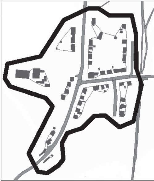
FIGURE 2. A ShrinkWrap Hull (the thick black line surrounding the buildings) (Revell. 2004)
